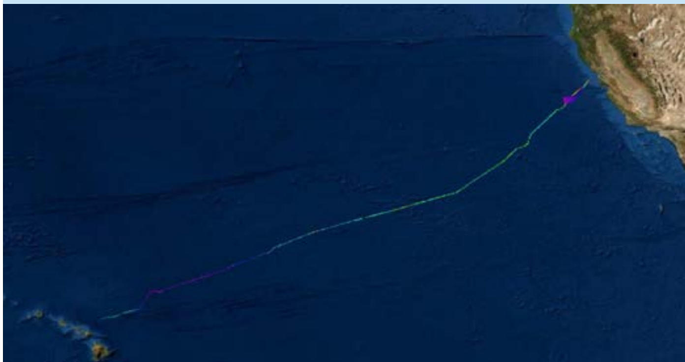
Multibeam data collected across the Pacific by an uncrewed system transiting from San Francisco to Hawai‘i Figure credit: Larry Mayer, University of New Hampshire
