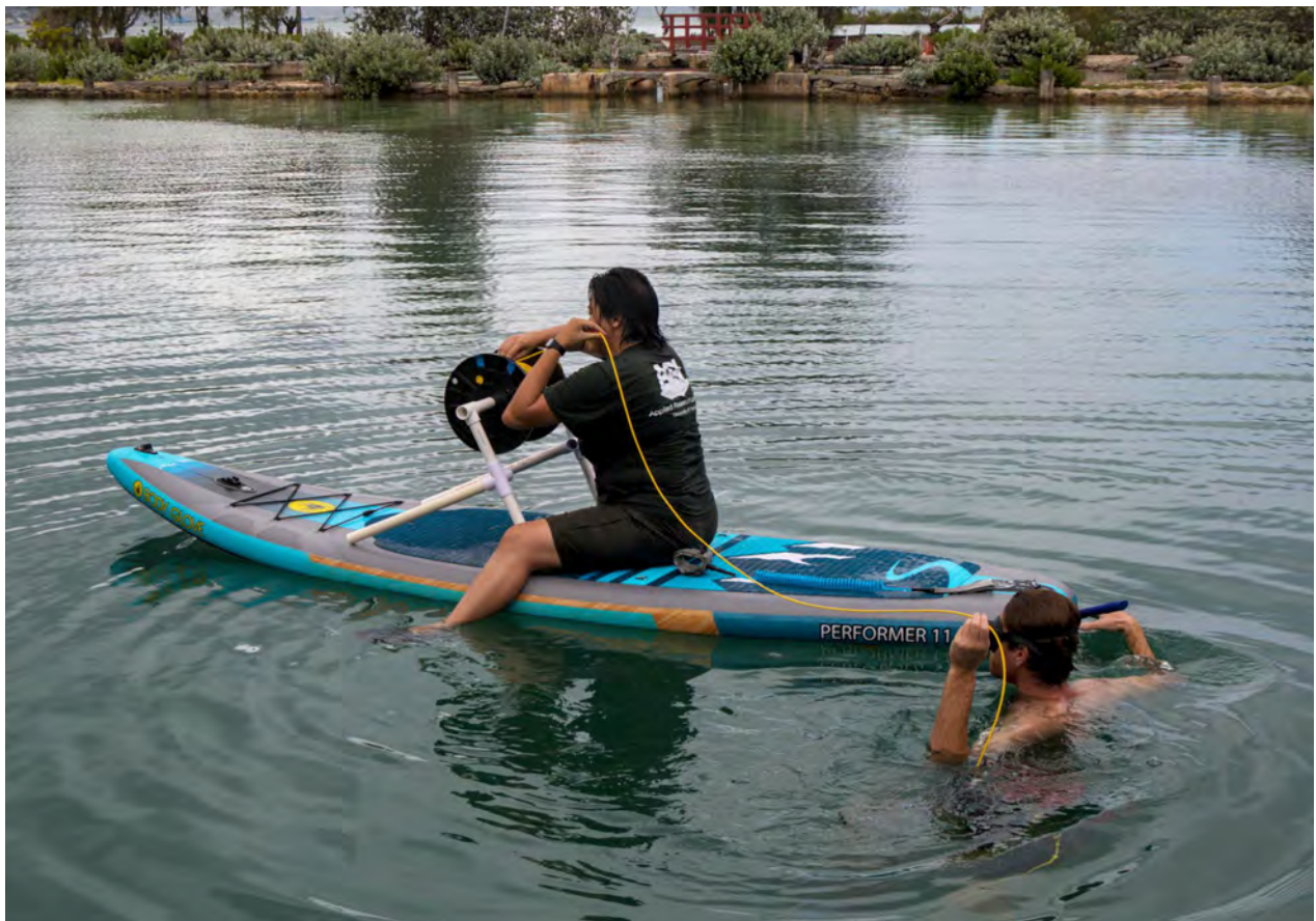
Figure 7: Deploying a fiber-optic cable into the small boat harbor at Moku o Lo'e.
